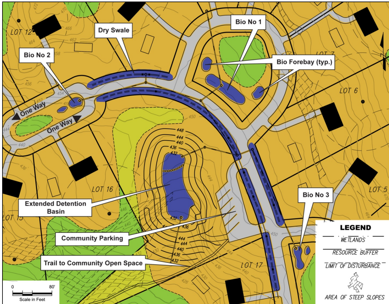
Figure D-3 Reaper Brook Estates Stormwater Management Controls – Plan View
